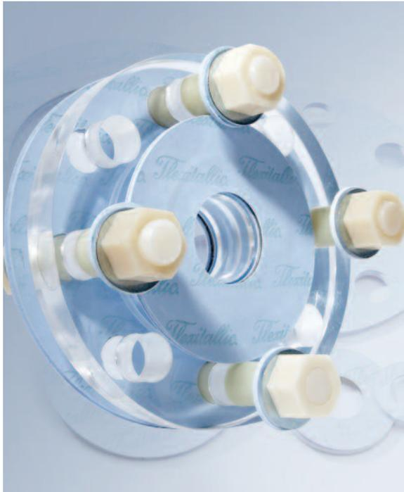
I-Flex electrical isolation systems are comprised of a main isolation gasket in combination with bolt isolation washers and sleeves. The main gasket is constructed from solid metallic core machined on upper and lower contact surfaces with Flexitallic's specially designed serration profile. The core surfaces are faced with structurally modified PTFE based on Flexitallic's proprietary Sigma® technology.
